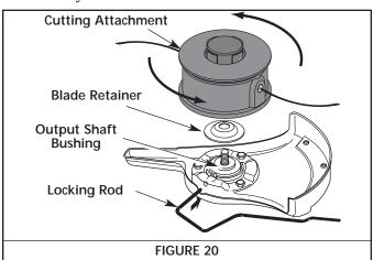
NOTE: The blade retainer must be installed on the output shaft in the position shown for the cutting attachment to work correctly.
